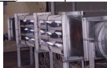
Fig. 9. A 36-electrode GlidArc pilot for VOC removal from exhaust.
