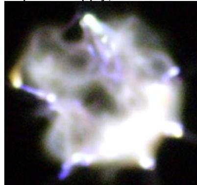
Fig. 3. Front view of GlidArc cold plasma generated between six electrodes.
