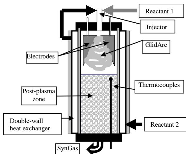
Fig. 7. Principle of the double-zone GlidArc reactor for POX reforming
