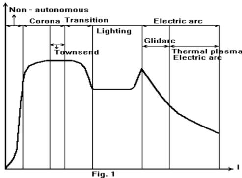
Fig. 1. General shape of Volt-Ampere characteristic of electric discharges in gases. One can observe that GlidArc is an autonomous discharge situated between the luminescent discharges and the electric arc.
