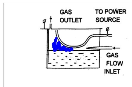
Fig.12. Gliding discharge between metallic and liquid electrodes.
