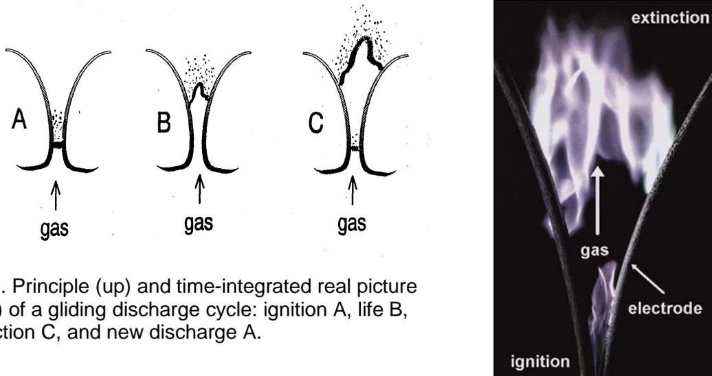
Fig. 2. Principle (up) and time-integrated real picture (right) of a gliding discharge cycle: ignition A, life B, extinction C, and new discharge A.
