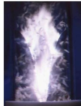
Fig. 11. GlidArc discharge in a spouted bed.
