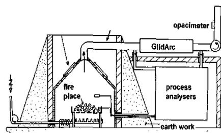
Fig. 10. Explosion-proof pilot plant for burning old munitions.
