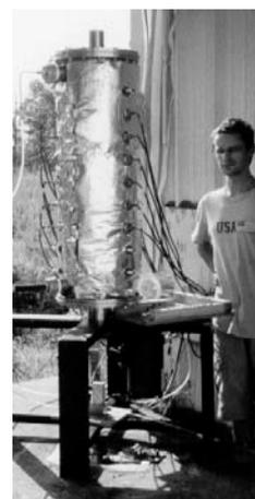
Precise mass and energy balances show that such acid gas processing (called SulfArc) can reach the H<sub>2</sub>S conversion rate of 99 % providing the Hydrogen and Carbon Monoxide (Synthesis Gas) at a quite low energy consumption.
