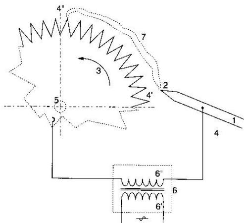
Fig. 4. Principle of the GlidArc-II device: 1 – stationary electrode, 3 – rotating electrode, 6 – power supply, 7 – high-voltage discharge.
