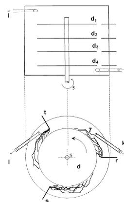
Fig. 5. Multiple-stages and multiple-electrodes GlidArc-II reactor: r, s, and t – three-phase-supplied stationary electrodes, k and l – input and output of the processed gas, d – rotating electrodes.
