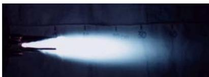
Fig.13. High-velocity flame of 60 kW (LHV) thermal power assisted by a 3-electrode GlidArc.
