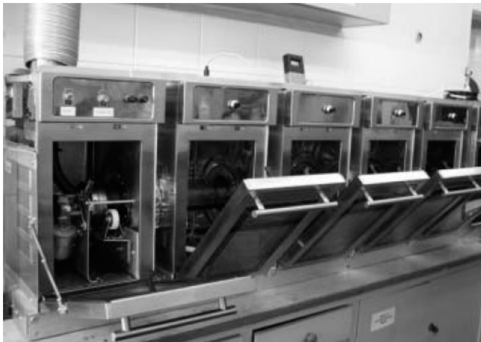
Fig. 3. Continuous MW polymerization reactor set-up at Cracow University of Technology
