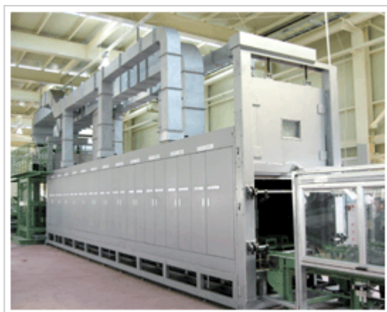
Fig. 2. Industrial microwave oven for continuous drying operations
