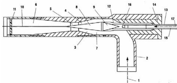
Fig. 1. Supersonic Gas-Liquid Reactor with two-phase flow patented by Praxair.
