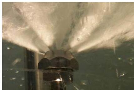
Fig. 2. Supersonic Gas-Liquid Reactor with gas nozzle submerged in liquid pool, developed at DSM.
