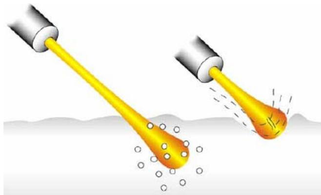
Fig. 3. Praxair's CoJet technology (left) and simple supersonic jet (right)
