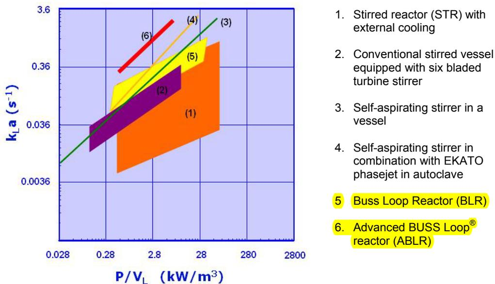
Fig. 3: Mass transfer rates in various reactor systems vs. power input per unit volume.
