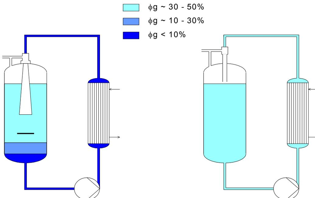
In the “classical” Buss Loop Reactor (built in the last 50 years), the gas was separated from the liquid in the reaction vessel and brought back to the head space, before entering the circulation pump.
