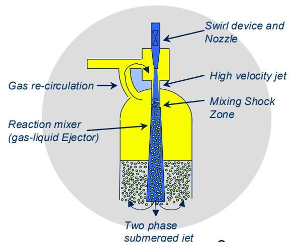
This creates intensive mixing shock zone where the high turbulence produces a fine dispersion of bubbles. The ability to generate and finely disperse very small gas bubbles to the liquid (30 to 70  $\mu\text{m}$ ) with a gas-liquid ratio between 0.5 and 2.0, or even more, makes this an ideal tool as primary dispersion device for gas-liquid reactors. The two-phase mixture created in the reaction mixer is then injected into the fluid of the reaction vessel.
