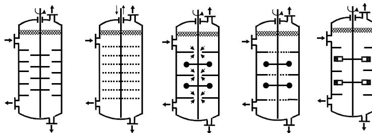
Fig. 2: Agitated columns (l.t.r.: RDC, Karr, Oldshue-Rushton, Kühni, Scheibel extraction columns)
