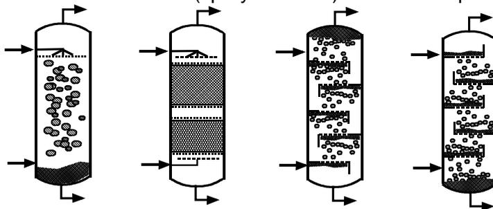
Fig. 1: Non-agitated columns (l.t.r: spray, packed, sieve tray (light) sieve tray (heavy) column)
