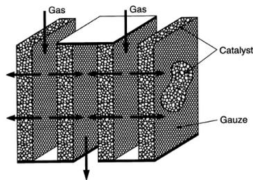
The gas passages in the LFR (Fig. 17) are each closed off at one end, neighboring passages being open and closed off at different ends. Thus, the gas is forced to flow through the layers of catalyst particles. The LFR found application in flue gas cleaning.
