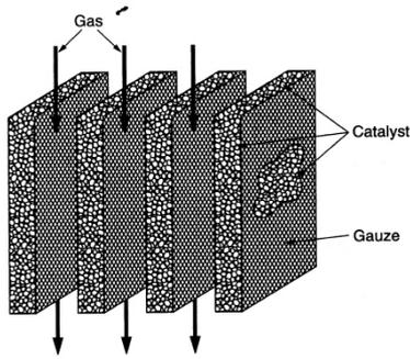
Fig. 15. Parallel-passage reactor
