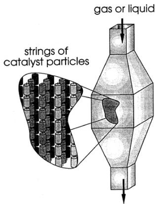
The B-SR (see Fig. 16) represents the limit of the PPR. The B-SR contains single-catalyst-particle subunits. Conventional particulate catalyst is fixed on parallel strings that are arranged parallel (or cross) to the main flow of reactants. The B-SRs have the advantages of the LFRs without the disadvantages of the LFRs (low mass transfer rates). Monolith with channels that are packed with the catalyst particles are in fact a kind of the B-SR (Strangio et al., 1999).
