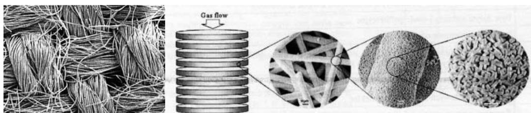
Fig. 9. Woven active carbon fiber catalyst      Fig. 10. Fibrous sintered metal structured catalyst arranged in layers
