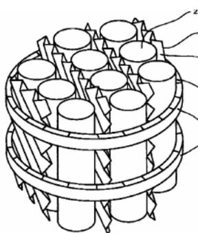
BASF AG has also developed a packing that has catalyst-holding and catalyst-free zones. The catalyst-holding zones are formed by hollow cylinders, open at the top and closed at the bottom, aligned along the column vertical axis. The cylinder walls are permeable to the reaction mixture, and impermeable to the catalyst. Structured separation layers (made from corrugated sheets) are in the catalyst-free zones, and the packing is held together by edge deflectors. The packing is shown in Fig. 14.
