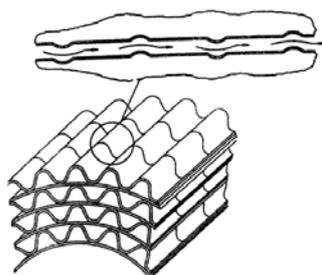
Fig. 1. EMITEC structure type TS
