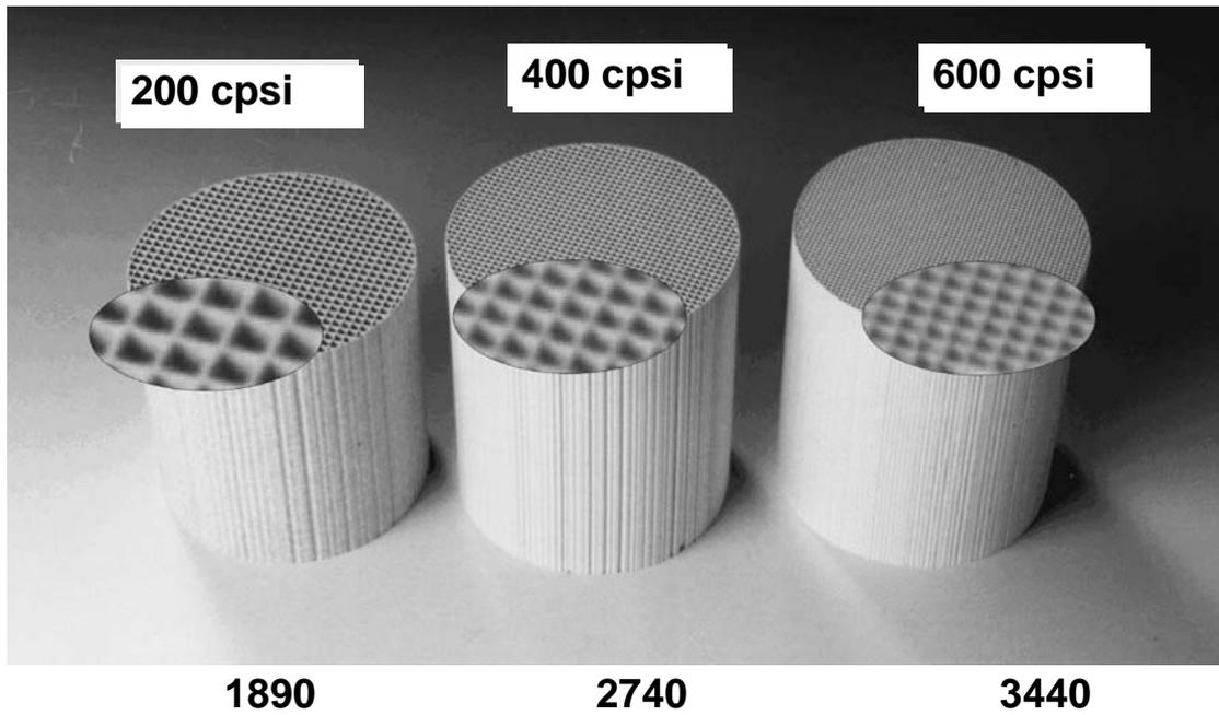
Fig 1. Typical examples of monolithic catalysts with different cpsi (cells per square inch). The numbers below the monoliths represent the volumetric surface area ( $\text{m}^2_{\text{geometric}}/\text{m}^3_{\text{reactor}}$ ).
