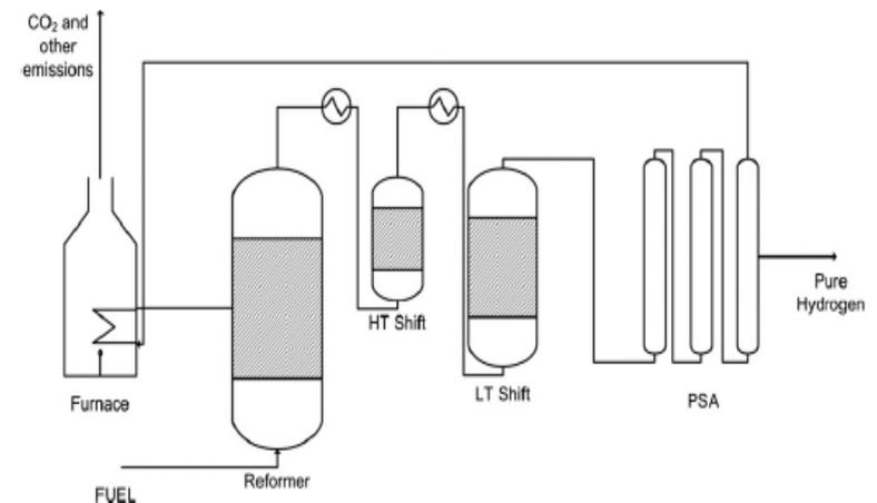
High temperature reformer, HT and LT shift, separations
