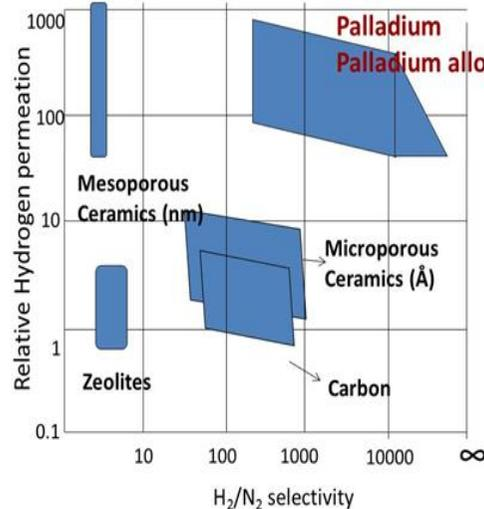
Pd alloys, thin layers 1-5 μm, supported by microporous ceramics
