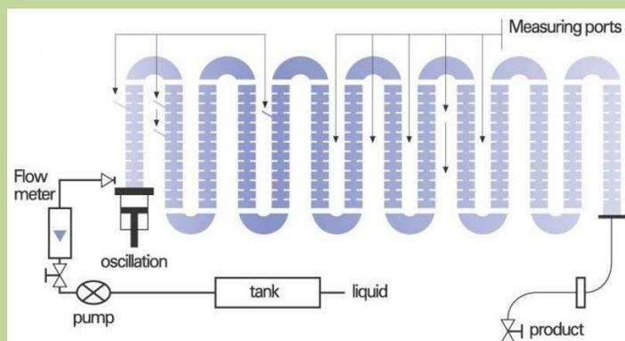
**OBFC** consists of a tubular crystalliser through which the mixture is pumped continuously that has to be crystallised.
