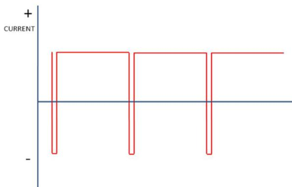
By applying pulsed current, the positive part of the current can be up to 10 times higher than 100% direct current. The negative spikes cause the polarization to become negligible.
