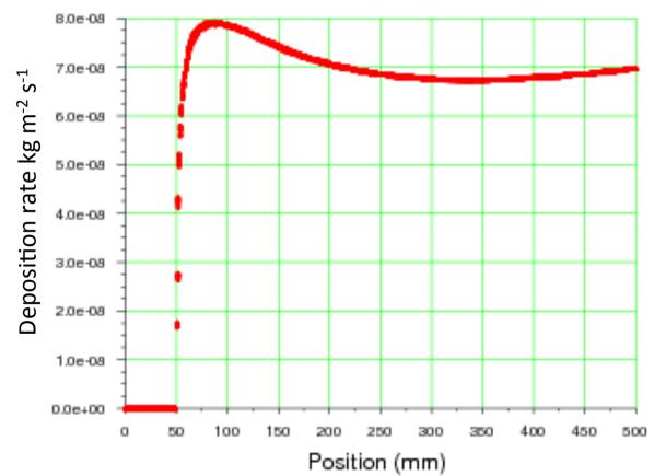
The predicted rate of coke deposition was similar to that observed experimentally
