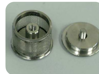
Basket agitator for handling catalyst
